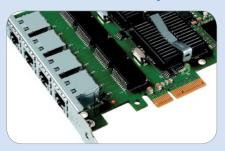
PCI Express<sup>3</sup> is designed to provide faster Ethernet network performance for desktop and server slots than that of PCI and PCI Extended (PCI-X). PCI Express derives a performance advantage from serial bus architecture that supports dedicated, bidirectional I/O at 2.5 GHz, compared to the 133 MHz parallel bus supported by PCI-X.
